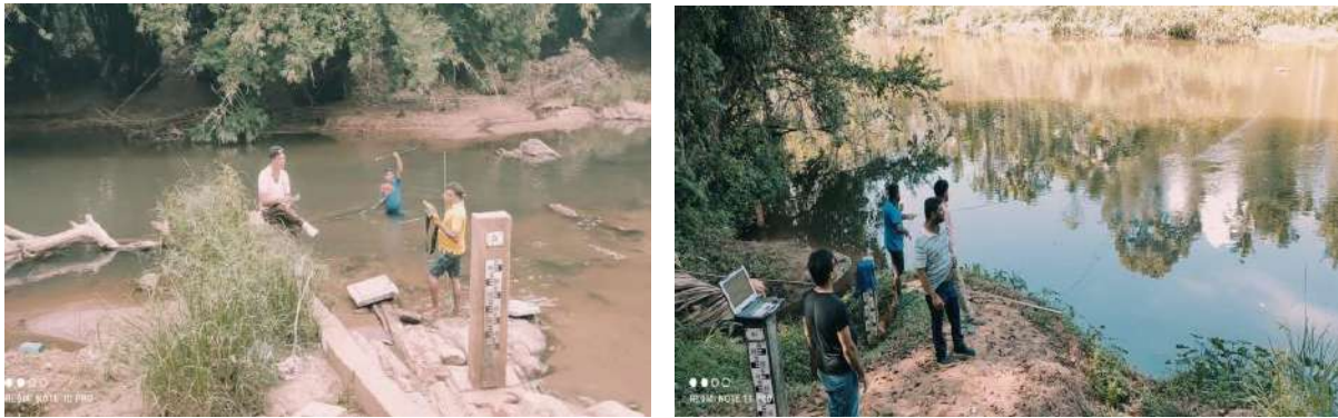
Figure 4-5: Current Metering at Kithulgala and Weweldeniya
