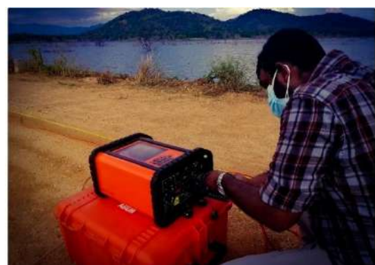
Figure 4-32: Resistivity surveying at Waththedara Morana
