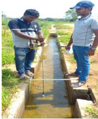
Figure 6-12: Fixing gauges & calibrate at Pavatkulam, Vavuniya
