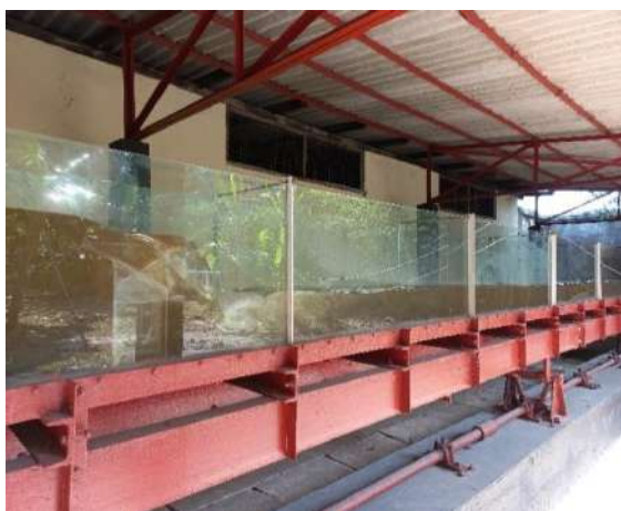
Figure 6-45: Experimental set up in 12.5 m long glass flume at Hydraulics Research Laboratory
