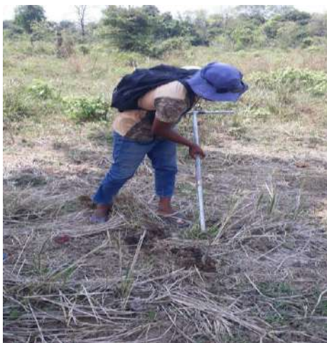
Figure 4-44: Examining the soils in Mundeni Aru river area of basin project using a bi-partite type augur
