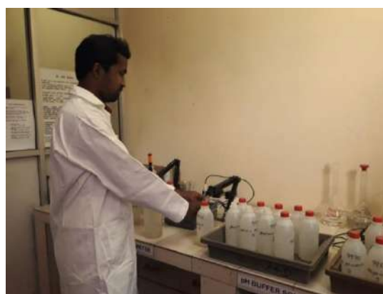
Figure 4-47: Analyzing water samples for pH and Electrical conductivity Spectrophotometer
