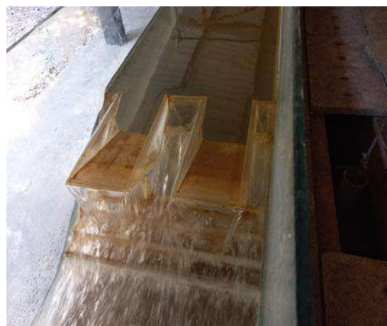
Figure 6-46: Flow over the PKW scale model of 1:20
