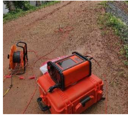
Figure 4-29: Resistivity surveying at Kelani Flood bund
