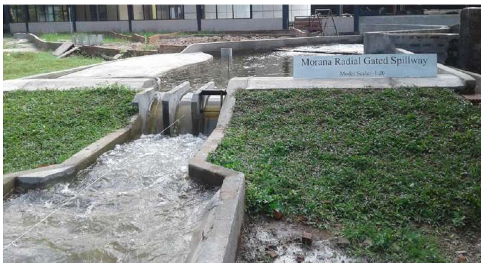
Figure 4-33: Completed model of Morana radial gated spillway
