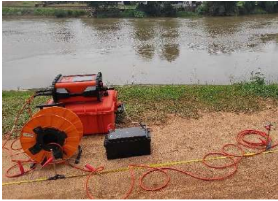
Figure 4-29: Resistivity surveying at Kelani Flood bund
