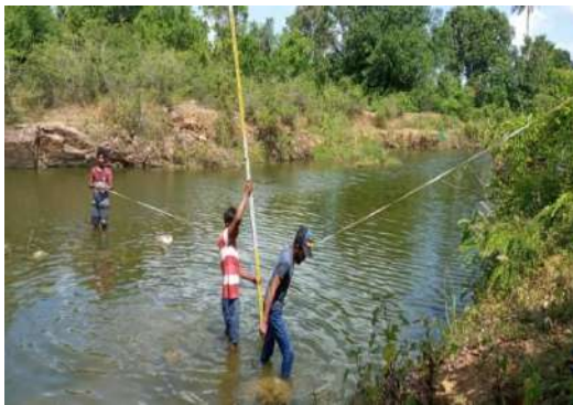
Figure 7-1: Surveying of River profile of Ma-Oya
