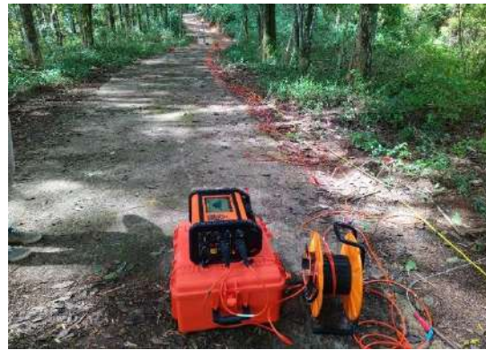
Figure 4-31: Resistivity surveying at Ambuluwawa
