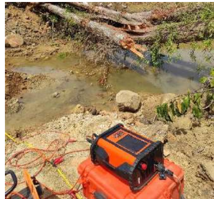
Figure 4-30: Resistivity surveying at Waththedara Bund Axis
