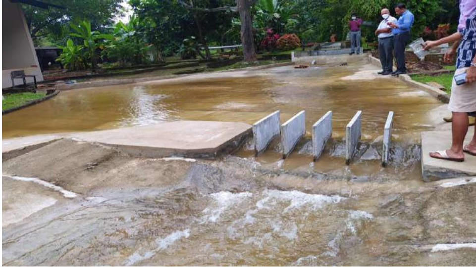
Figure 4-34: Existing condition - Mavadiodai Anicut model
