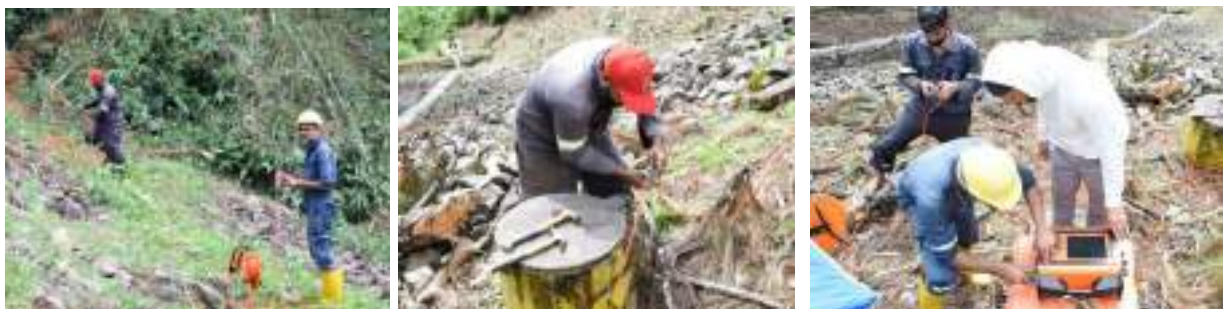
Figure 4-4: Resistivity survey at Maussakele saddle dam
