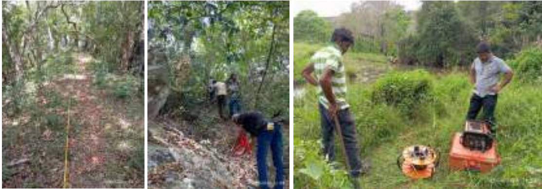
Figure 4-3: Resistivity survey at Thalapathkulama
