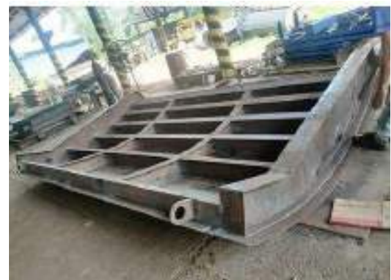
Figure 8-11: Magallagoda Gravity Gate Refabricating and Installation works by Regional workshop Halpathota
