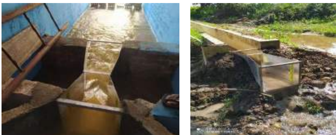
Figure 4-15: Calibrating Cutthroat flume at HRL
