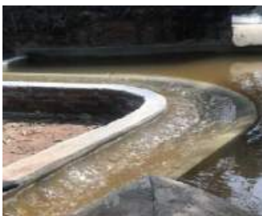
Figure 4-12: Model testing of Ellewewa uncontrolled chute spillway
